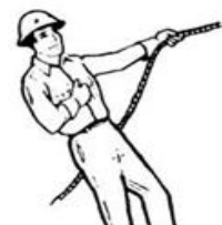
EXTEND BOOM (Telescoping Booms)
