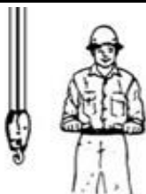
RETRACT BOOM (Telescoping Booms)
