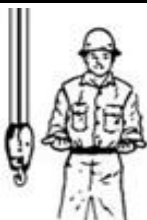
EXTEND BOOM (Telescoping Booms)
